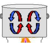
Heated water rises from the bottom to the top of the pot. Cold water replaces the rising water.
